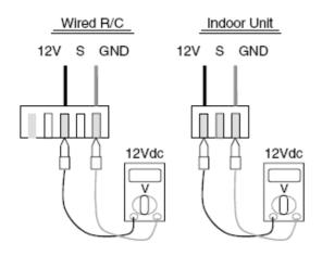
The Red cable is 12 Vdc The Brown or Black cable is Ground or 0 Vdc The Yellow is signal (Comms.)
