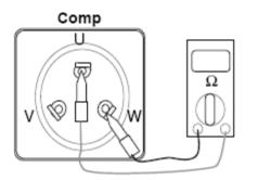
Disconnect the electrical connections to the compressor and check the resistance of the compressor windings, measure from U to V, V to W and W to U the values should be between 0.25 and 5 Ohms each.
