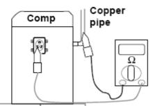
The next test is to measure the resistance of the compressor windings to earth. Using a Megger (High Voltage Meter) measure the resistance from any of the 3 compressor terminals to an Earth point (pipe work).
